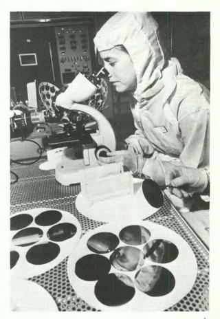
MELAINE TUCK (2141) views photolithographic patterns on silicon wafers through a microscope. Below, she places in-process silicon wafers in a dry nitrogen storage cabinet. The dust/lint protective clothing is worn by all employees working in the clean room area.
